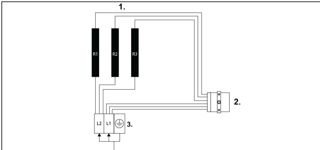
**1**= Heating elements **2**= Overheating limit control **3**=Ground
