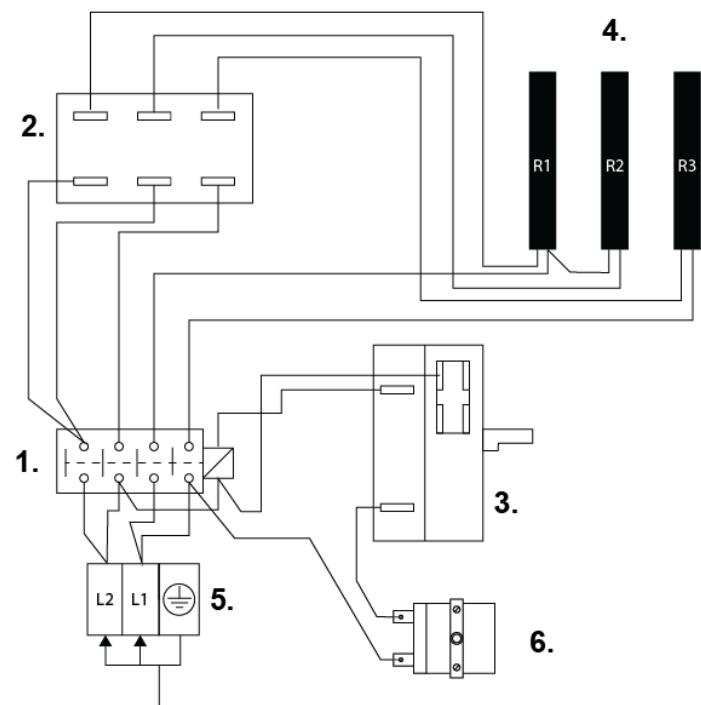
1= Contactor 2= Thermostat 3=Timer 4=Heating elements 5=Ground 6= Overheating limit control
