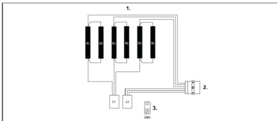
1= Heating elements 2= Overheating limit control 3=Ground
