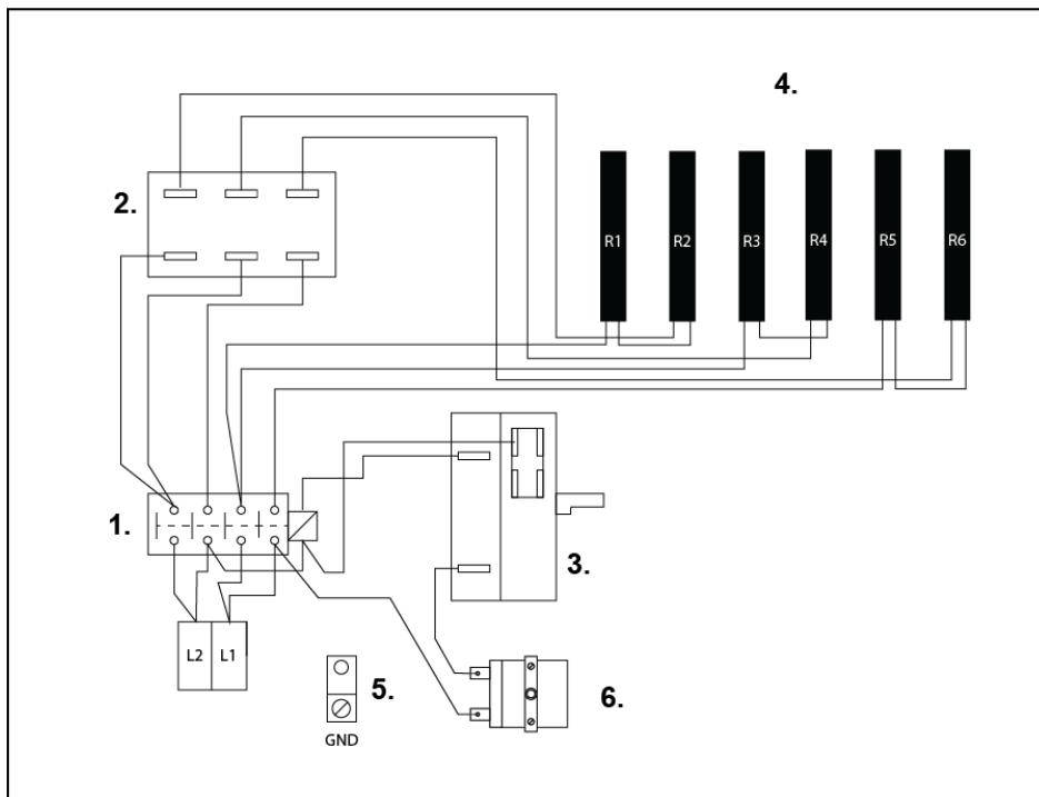
1= Contactor 2= Thermostat 3=Timer 4=Heating elements 5=Ground 6= Overheating limit control
